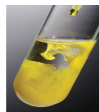
Figure 10.3 Precipitation of PbI_2
