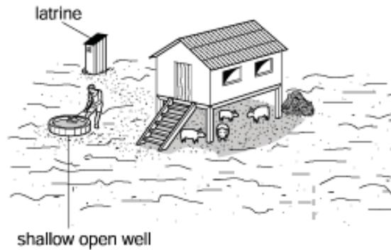
**Fig. 2: A Pit Latrine Located Very Close to a Water Source** (Cambridge International Examinations Science Diagrams for Examiners)
