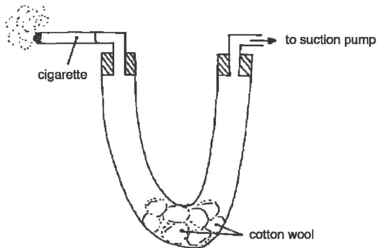
**Figure 3:** Experimental set up to demonstrate the presence of tar in tobacco smoke.
