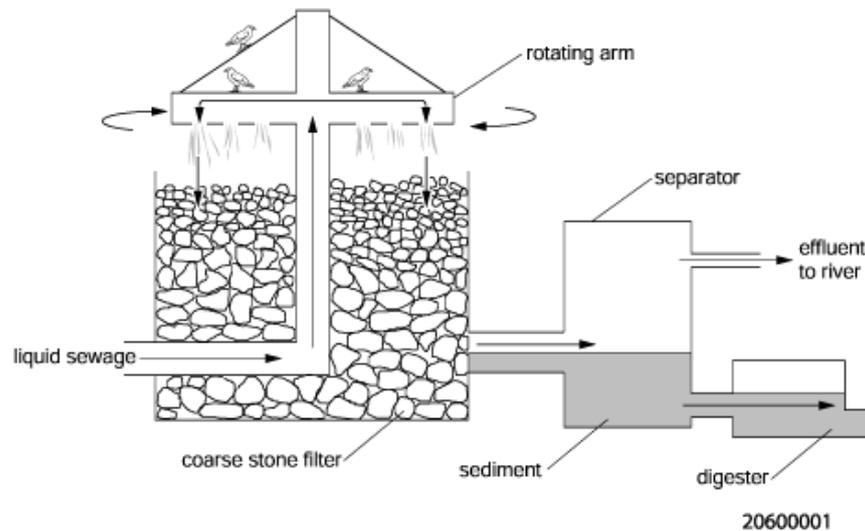
**Fig. 3: sewage trickle filter section** (Cambridge International Examinations Science Diagrams for Examiners)
