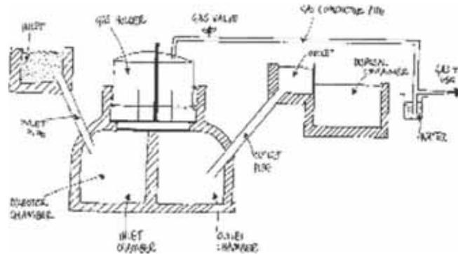
**Figure 2:** Equipment for the production of biogas
