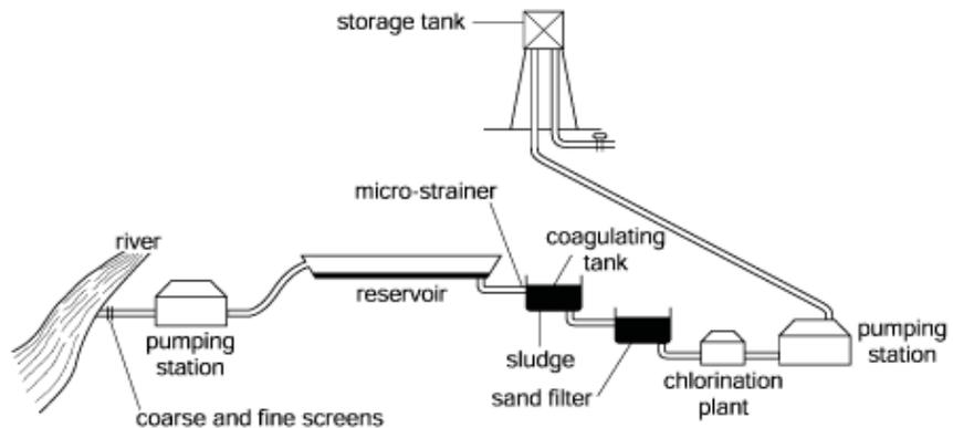
**Fig. 3: Water Works System** (Cambridge International Examinations Science Diagrams for Examiners)
